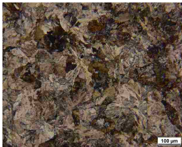
Figure 23 – LOM photomicrographs of Sample 4 from CF&I77 rail as viewed at the mid length of the sample.
