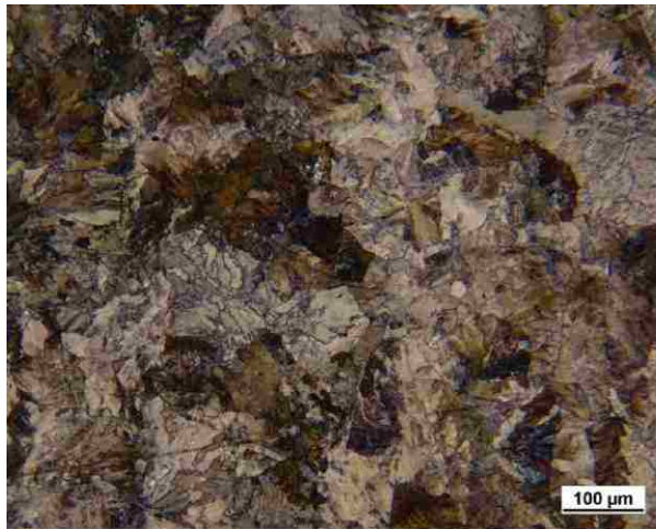
Figure 28 – LOM photomicrographs of Sample 4 from CF&I77 rail as viewed at the end of the sample.
