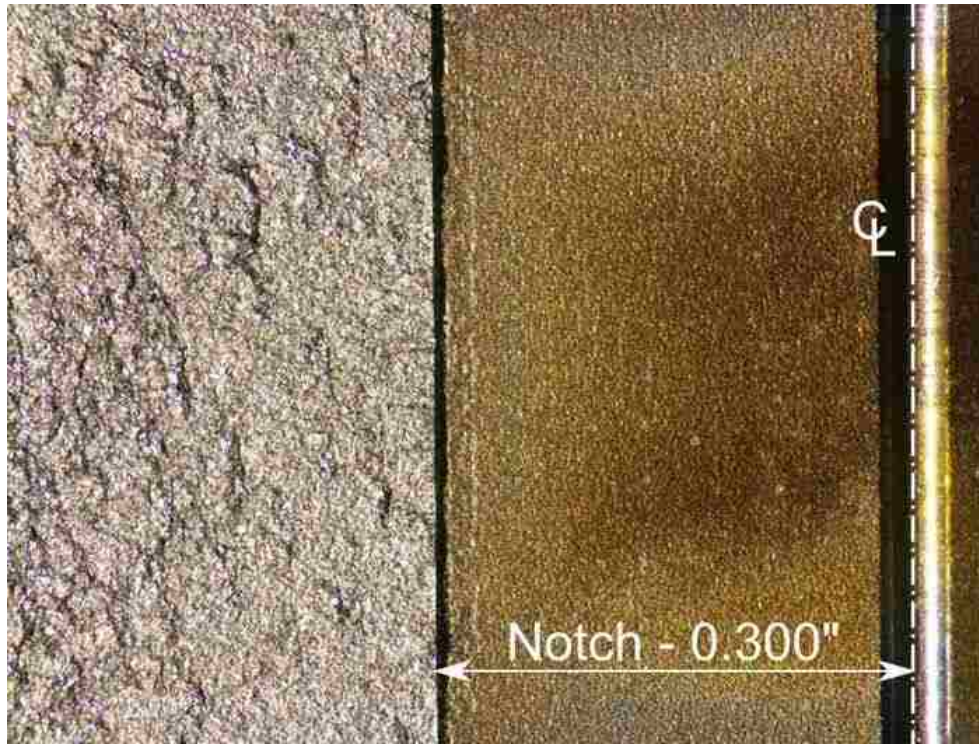
Figure 89 – Fatigue/fracture surface taken from HH rail CCT test specimen showing rough fatigue crack surface.
