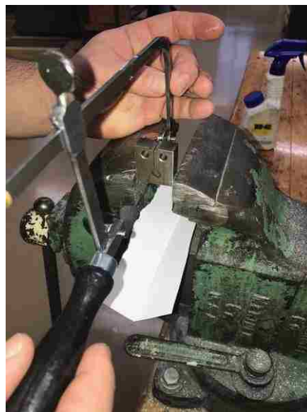
Figure 52 – Cutting sharp notch at the base of waterjet cut notch using jeweler's saw.
