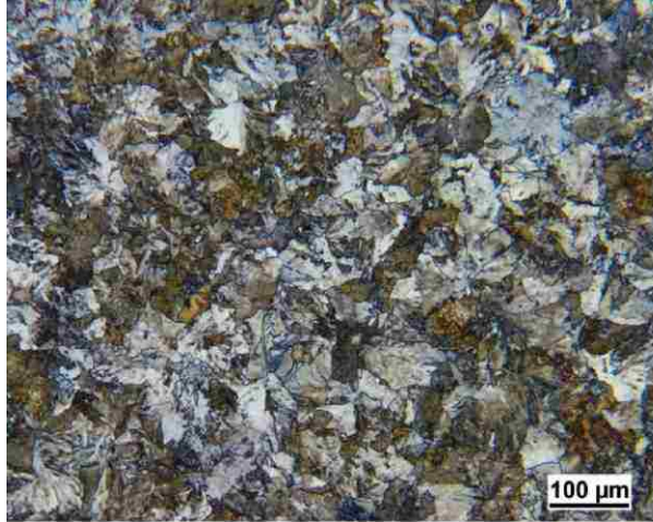
Figure 27 – LOM photomicrographs of Sample 4 from AHH rail as viewed at the end of the sample.
