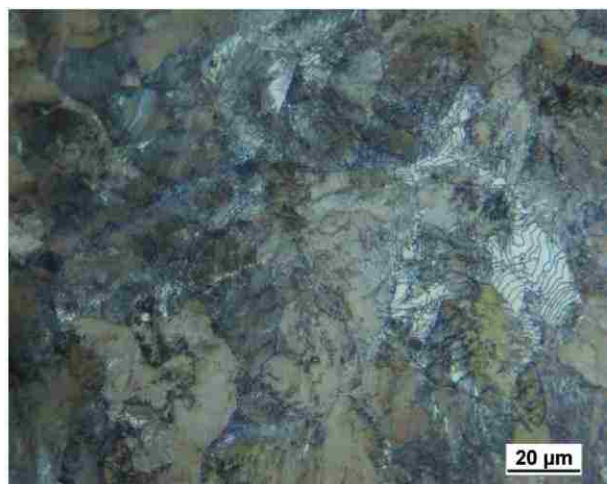
Figure 25 – LOM photomicrographs of Sample 4 from SS rail as viewed at the end of the sample.
