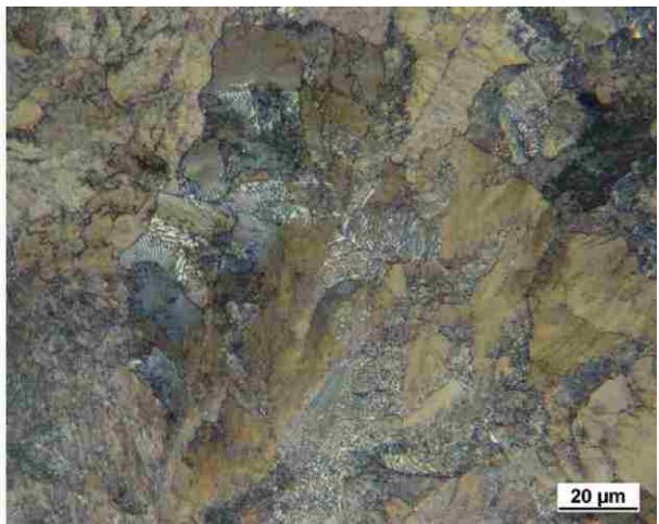
Figure 23 – LOM photomicrographs of Sample 4 from CF&I77 rail as viewed at the mid length of the sample.
