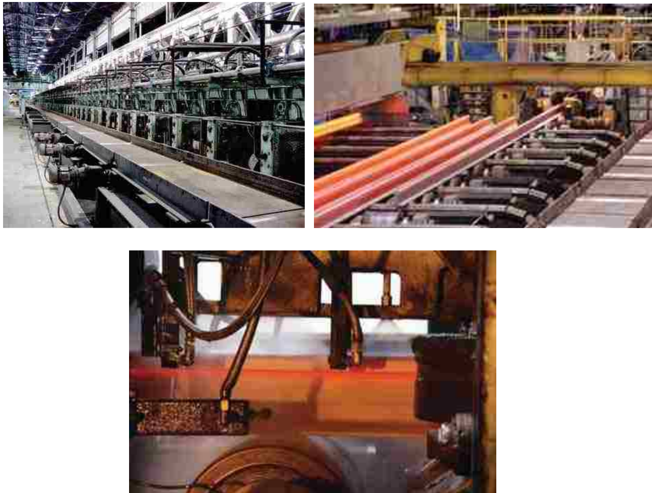
Figure 3 – Head hardening facility at ArcelorMittal, Steelton.
