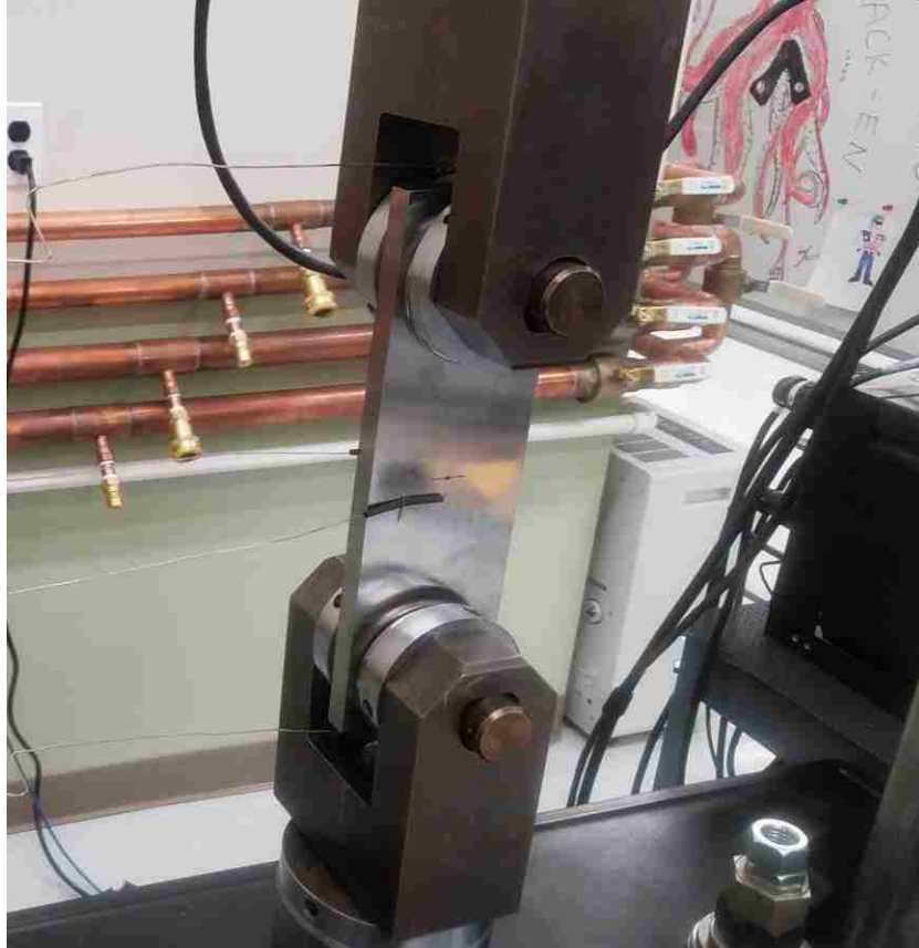
Figure 86 – Testing of center cracked tension (CCT) specimen at LTI.
